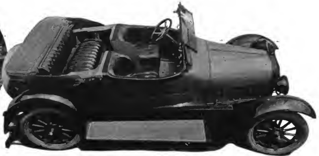
View of rear deck closed and opened for Anderson five-passenger roadster
